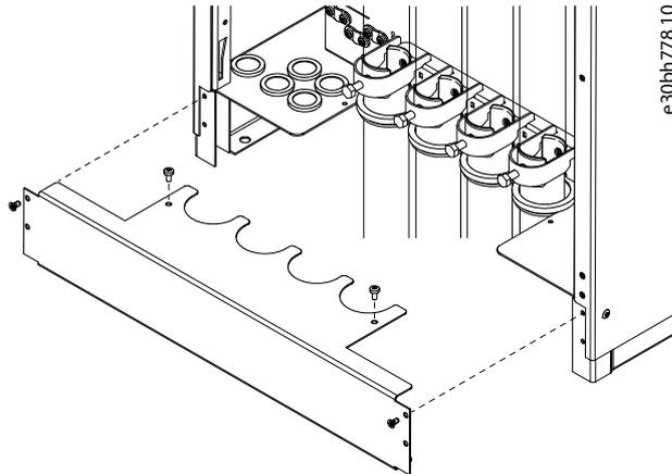
6. Attach the safety covers. For the tightening torques of the screws, see [12.5 Tightening Torques for Cover Screws](#). Make sure that the control cables or the cables of the AC drive are not caught between the frame and the safety covers.
