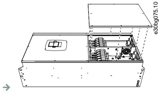
2. Find the DC terminals and Brake resistor terminals on top of the AC drive.
