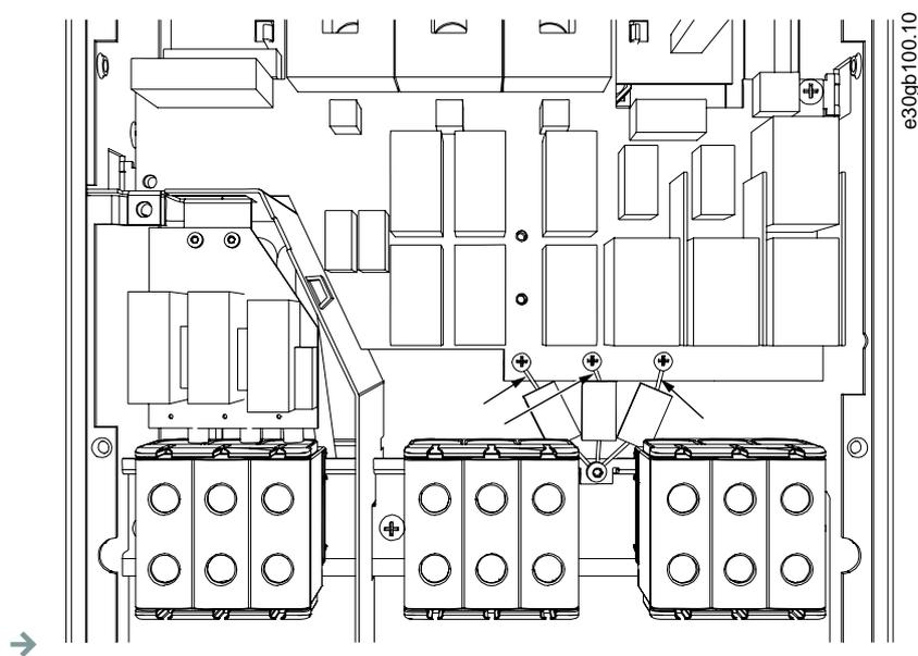
5. Remove the screw and the capacitor assembly.
