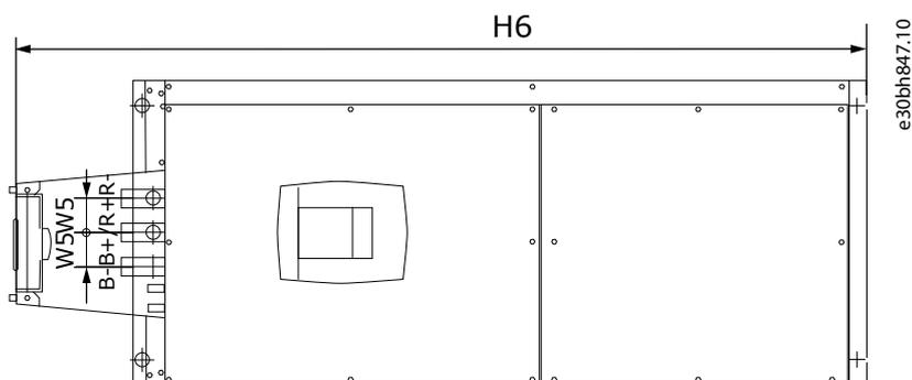
Illustration 67: Dimensions of the VACON® NXS/NXP AC Drive, FR9 with DC Extension Connection Box
