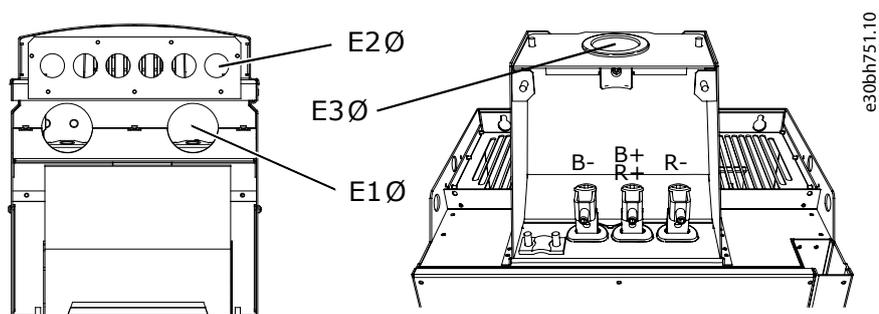
**Illustration 65: Dimensions of the Mounting Holes for VACON® NXS/NXP AC Drive, FR8**
