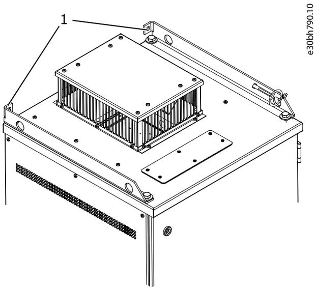
1 Fixing hole,  $\varnothing= 13$  mm (0.51 in)
