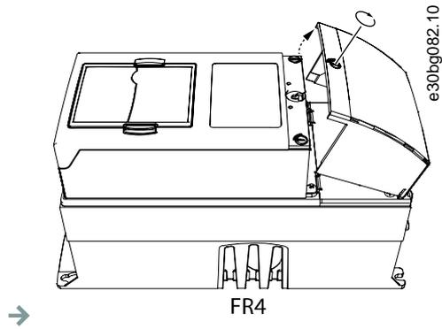
2. Remove the screws of the cable cover. Remove the cable cover. Do not open the cover of the power unit.
