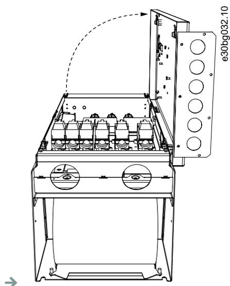
3. Find the DC terminals and Brake resistor terminals on top of the AC drive.
