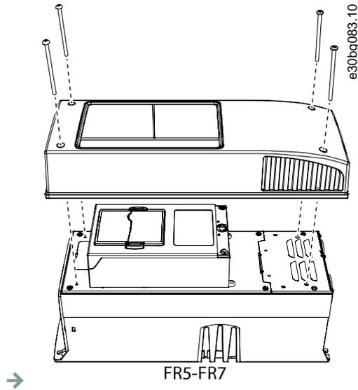
2. Remove the screws of the cable cover. Remove the cable cover. Do not open the cover of the power unit.
